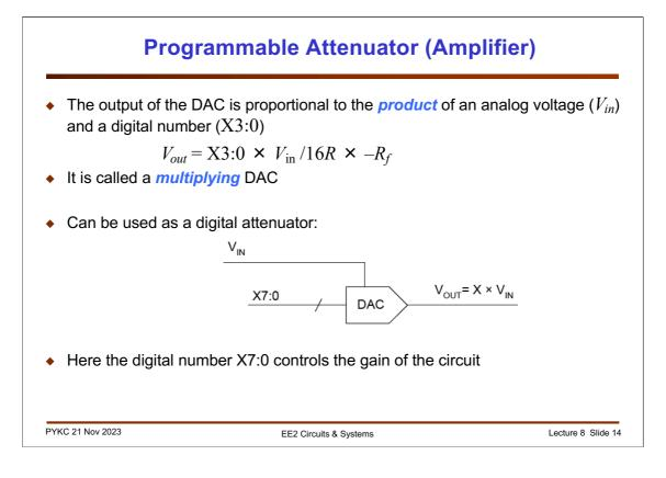
Instead of using Vref, a fixed reference voltage, we could use an analogue input Vin (such as an audio signal), and then use the DAC as a digitally control amplifier or attenuator. This is also known as a multiplying DAC. The output is X multiplied by Vin.
