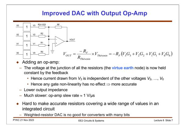
The high output impedance of the previous circuit can be circumvented using an operational amplifier. Shown here is a summing amplifier. Vout is given by this simple linear equation. The output impedance is that of the op amp and is very low.
