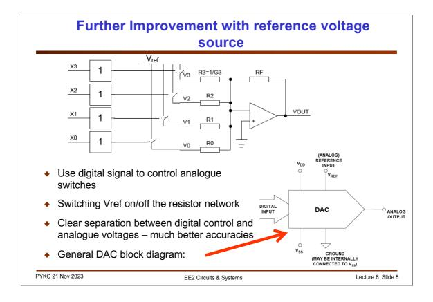
Instead of driving the resistor network directly from the digital output, which is not very accurate, most DAC actually use the digital signal to control electronic switches which switch in or out a reference voltage Vref. This reference voltage can be made very accurate, thus providing accurate output voltage values.
