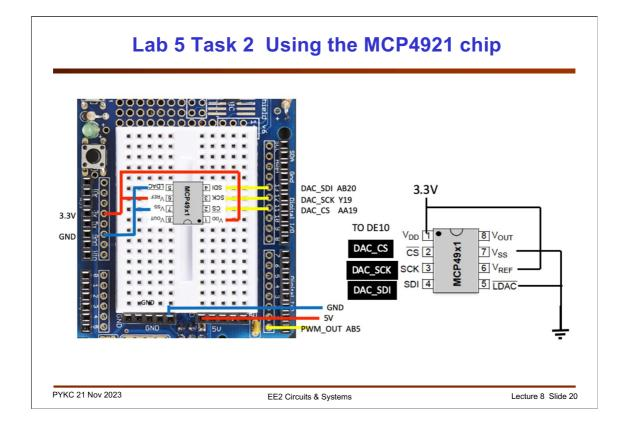
Lab 5 Task 2 requires you to add the DAC chip to the DE10 to produce directly the analogue output voltage from the digital input. The MCP4921 chip uses the SPI interface. A module spi2dac.v is provided. The detail working of spi2dac.v will be explained in a later lecture. For now, just used this as a given component.
