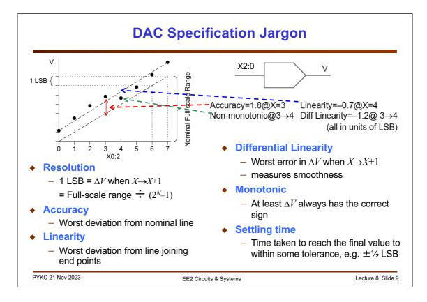
Here are the important specifications found in a datasheet that defines the performance of a DAC. Here we use the line from full range value to the origin as reference. We will express all voltage in terms of the delta-v corresponding to one LSB.
