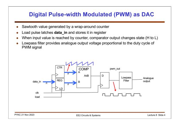
Here is a circuit schematic for a pulse-width modulated DAC. Here the counter is used to produce a count value A that ramps up linearly in a sawtooth manner. The digital value we want to convert to analogue value is data\_in, which is stored as B in the input register.
