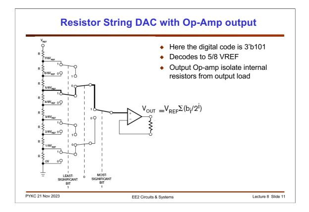
Instead of using a large number of switches, we can also use switches arranged in a tree structure as shown here. Here is an example showing the decoding of the digital value 3'b0101. Decoding is implicitly performed via the control of the switches using the three digital bits. The output op amp provides buffering of the DAC voltage.
