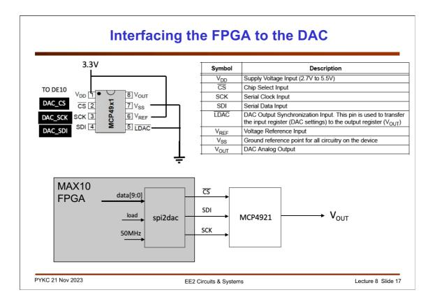
This is a simplified diagram showing how the MAX10 FPGA is interfaced to the MCP4921 DAC.
