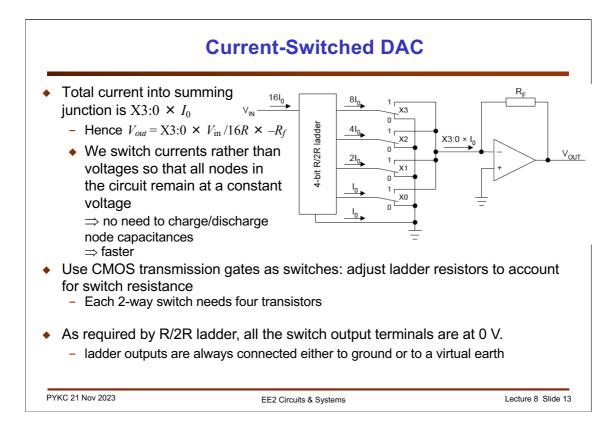
For a practical DAC circuit, the R/2R ladder network is connected to the virtual earth of the op amp as shown here. The current is either sent to the virtual earth node if the digital value is '1', or switched to earth if it is '0'. In that way, the output voltage Vout is a converter analogue value of X[3:0].
