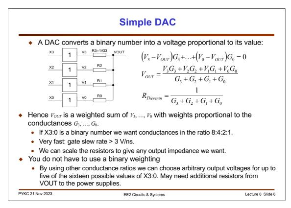
The simplest DAC can be constructed using a number of resistors with binary weighted values. X[3:0] is the 4-bit digital value to be converter to an analogue voltage Vout. The 4-bit number is used as input to buffer circuits (the rectangular blocks labelled '1'). The outputs of the four buffers are V[3:0] respectively.
