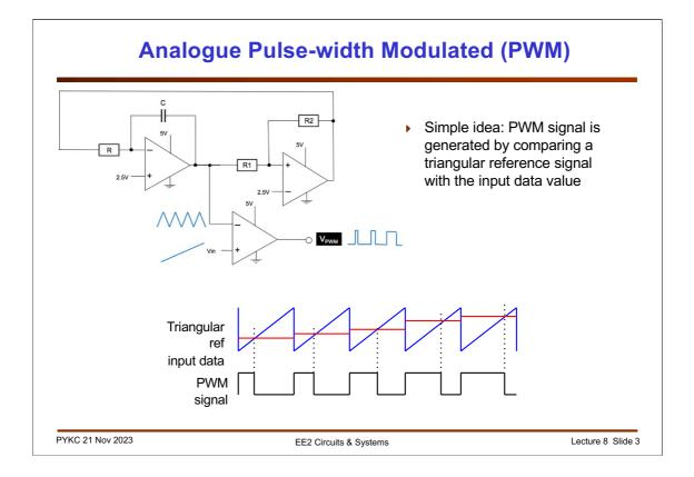
In Lecture 4, we explored the use of op-amps to build an analogue pulse-width modulator using an integrator, a comparator with hysteresis (also known as a Schmitt trigger circuit), and a simple analogue comparator.
