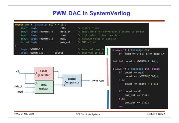
Implementing a PWM DAC is extremely simple in SystemVerilog. Here is the code with colour coding for the three major blocks.
