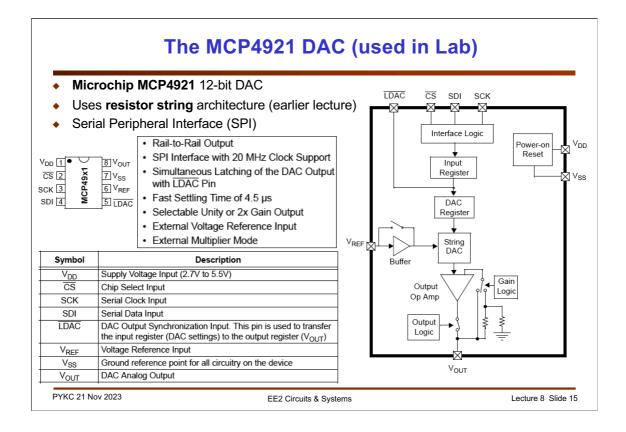
The DAC used in the lab experiment is 12-bit. However, since the accuracy of the DAC is only up to 10-bit, only the top 10 bits are used throughout our lab sessions.
