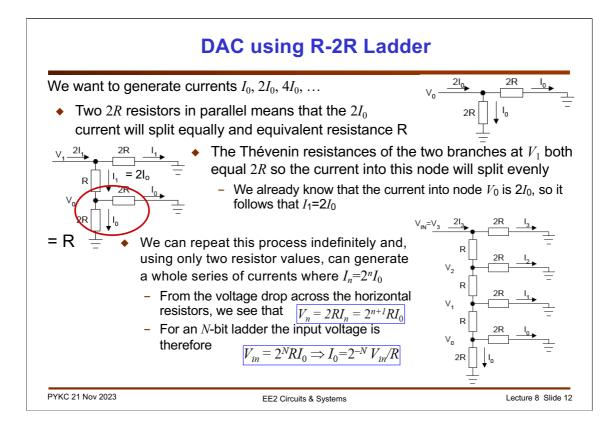
String resistor network is good for, say, up to 10-bit DAC (requiring 1024 identical resistors). If you want a 16-bit DAC, you would need 65536 resistors! That is obviously not practical or too expensive. A better solution is to use R-2R Ladder network.
