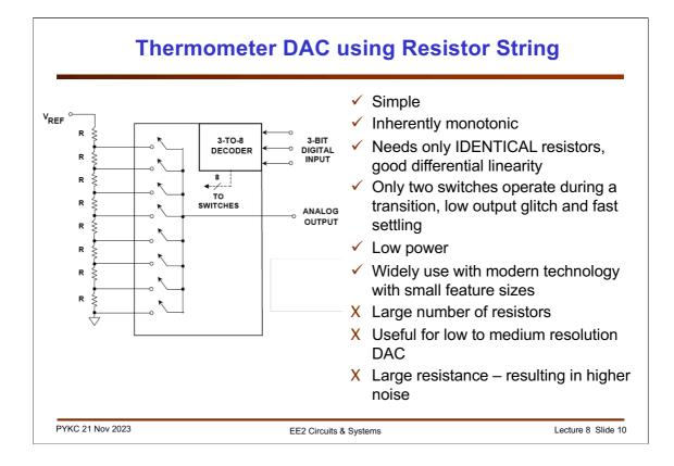
Instead of using binary weighted resistor network, we could use a series string of identical resistors as shown here. With this architecture, Vref to 0 is divided into 8 equal steps (including 0 value). The 3-bit digital input is decoded into 8 possible binary one-hot codes. For example, 000 results in the lowest switch being connected and 111 will switch the upper most switch on.
