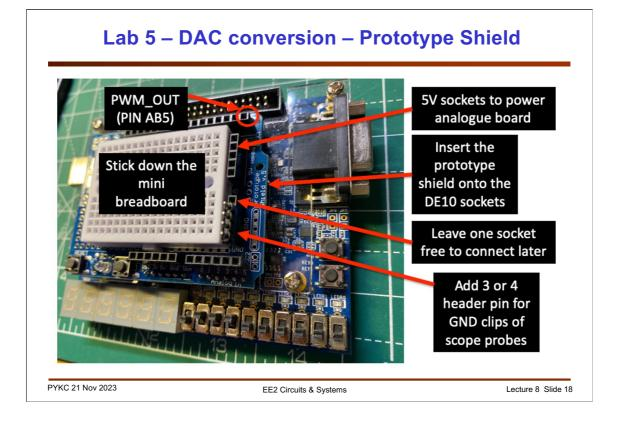
You will have a chance to try out the contents of this Lecture when you do Lab 5. Before you start, you need to add a prototyping add-on board (a shield) to the DE10-Lite module as shown in the slide here. You will then add on the breadboard the MCP4921 digital-to-analogue converter chip. Later in Lab 6, you will add another chip for analogue-to-digital conversion.
